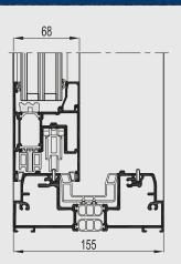
Concept Patio® 155 is a premium insulating slide and lift-slide system, designed to create maximal glass areas, combined with increased comfort. The sophisticated concept fulfils the user's high expectations of optimum quality, high insulation and ease of operation.
